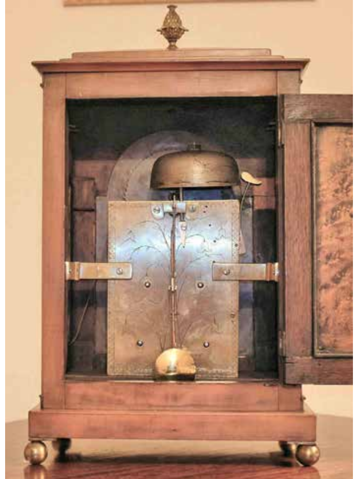
Figure 6. The anchor escapement and back plate engraving can be seen in this view.
