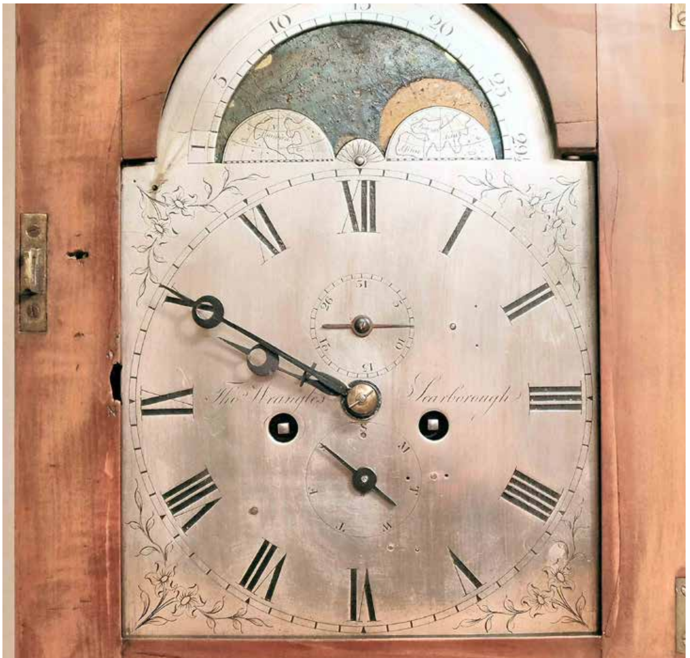
Figure 2. The single sheet brass dial is unusual, perhaps unique, for a bracket clock in displaying the calendar (day of the month) below XII and the day of the week by its initial letter above 'VI'. This indicates that the clock was made purposely as a one-off, not bought in as a standard item simply to be retailed by Wrangles.
