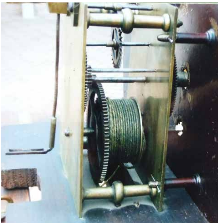
Figure 2. The movement, seen here from the left, has plates which are what we call 'A-shaped', though only slightly so. This is a typical feature of most tavern clocks.
