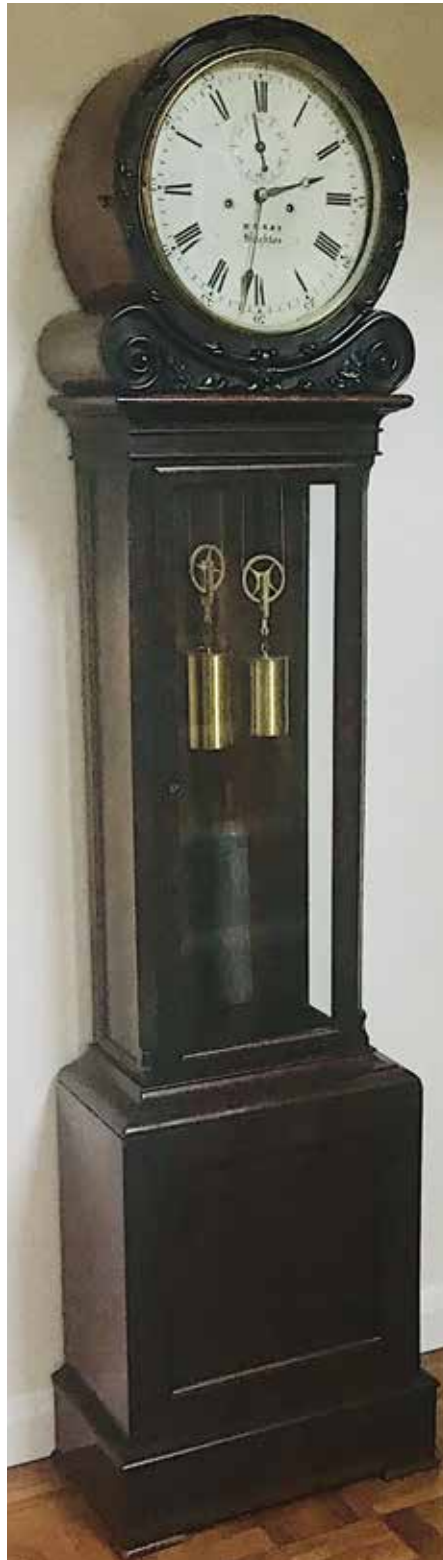
Figure 1 The shop regulator by W S Ray of Brighton was probably made about 1854, when he took over the business from his father. The mahogany case has a typical glass door to display the brass driving weights with spoked pulleys. This example strikes the hours.
