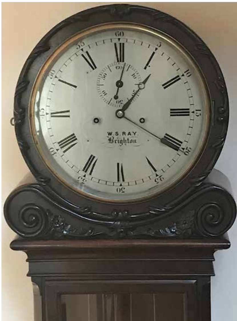
Figure 2. The silvered brass dial has conventional layout for the hands. The movement has a dead-beat escapement and Harrison's maintaining power. A hint of decorative carving to the mahogany cases gives the impression of a director's clock on a pedestal.
