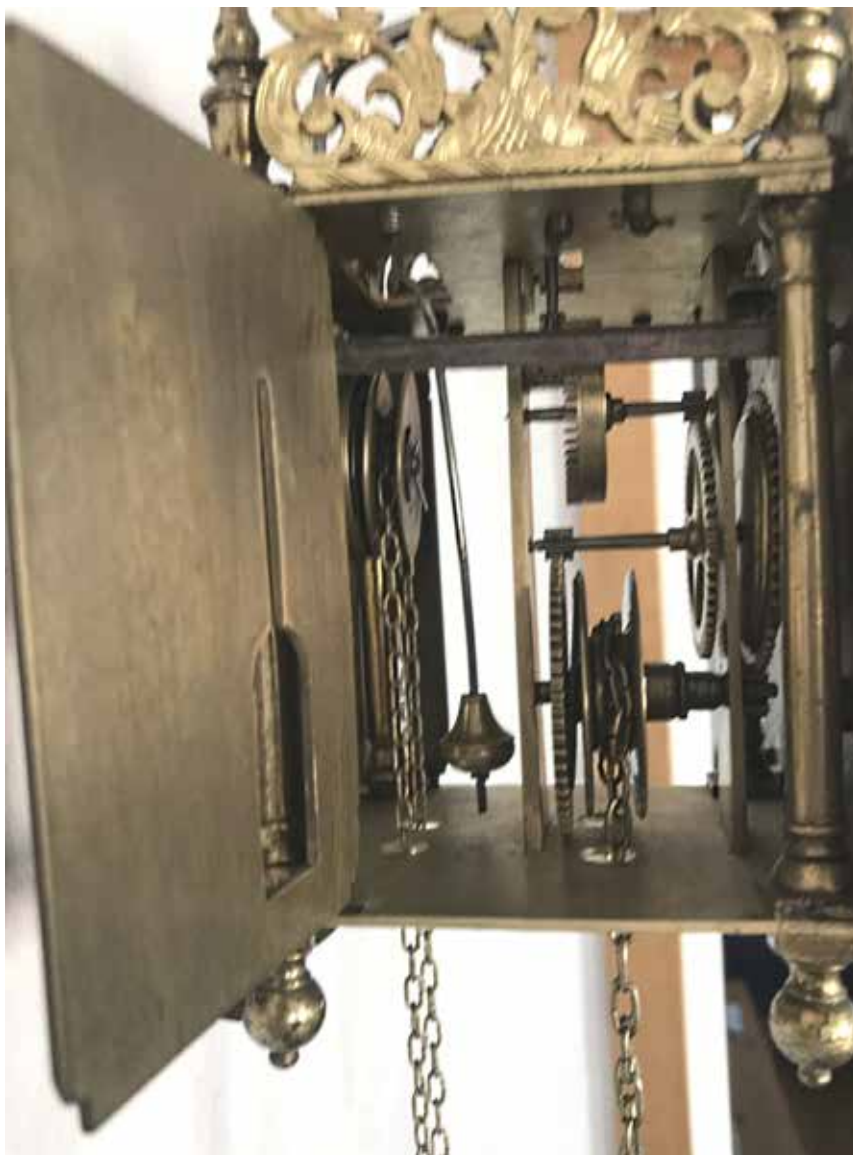
Figure 2. The movement from the left shows the verge escapement going train with alarmwork set on the backplate. Photograph by Olov Johanson.
