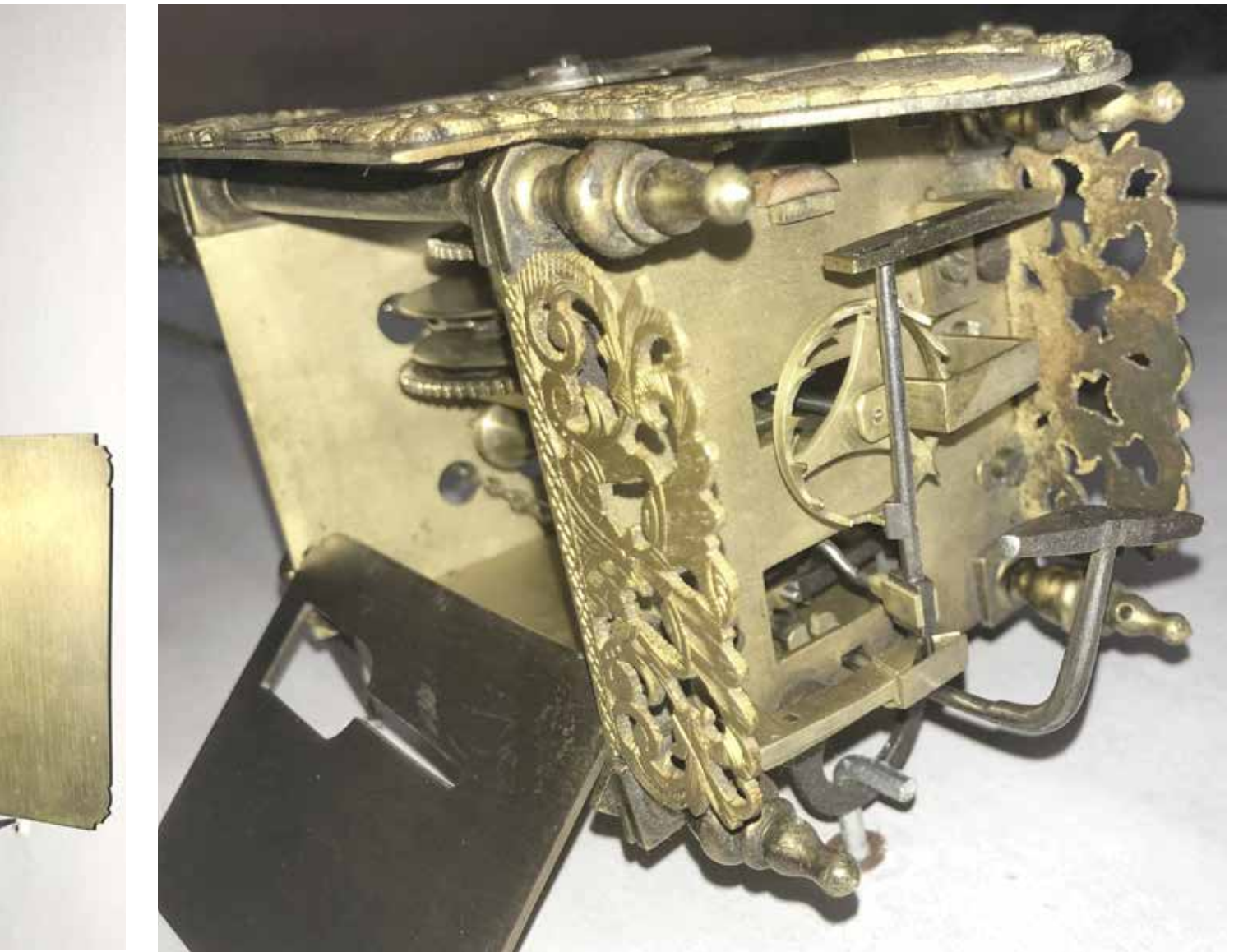
Figure 4. Full view from above showing the verge escapement in detail. Photograph by Olov Johanson.
