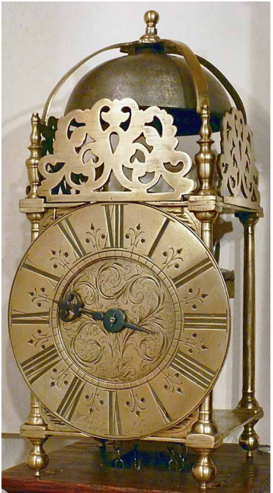
Figure 6. The same clock after cleaning. The hand has now been repaired correctly.
