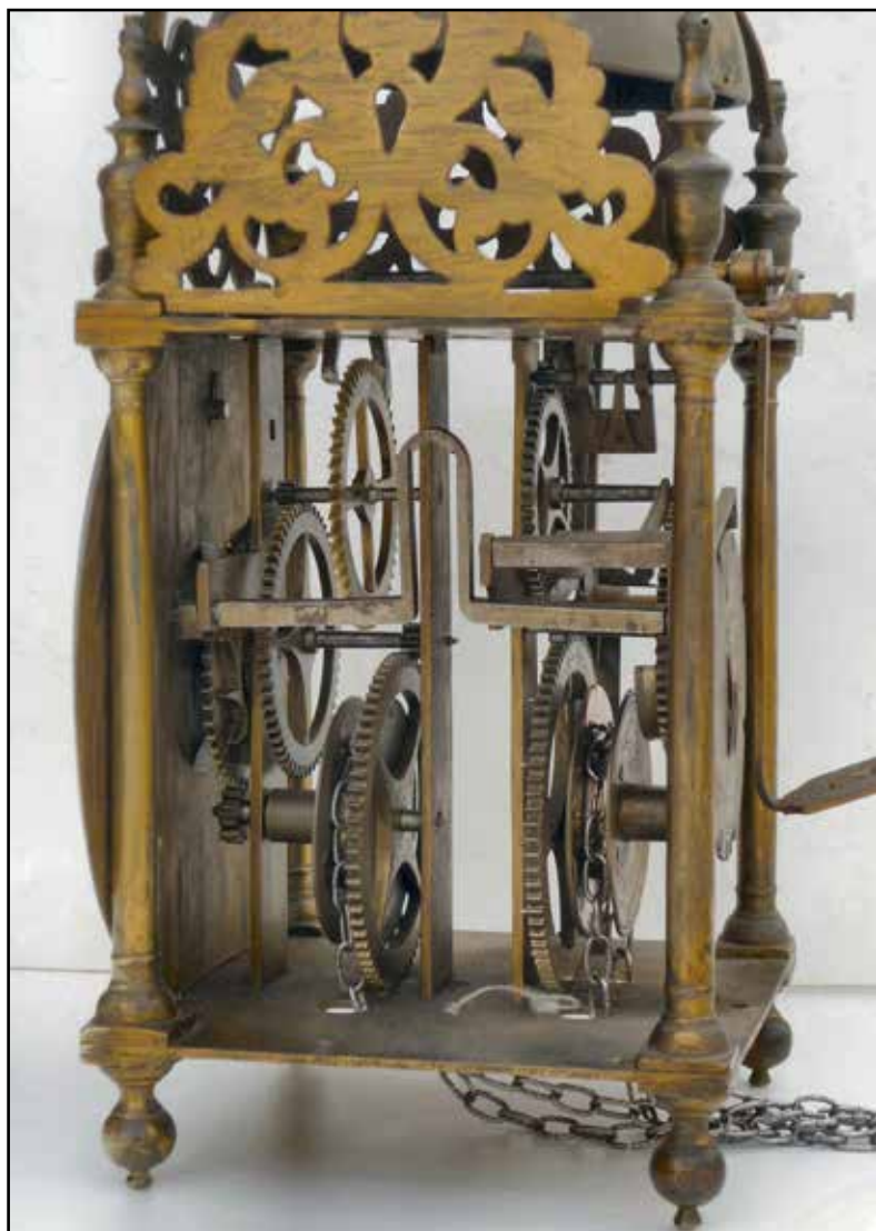
Figure 7. The movement of the Barlow clock before cleaning, showing the hammer spring with traditional filed decoration. The escape wheel has a different profile from the original wheels.
