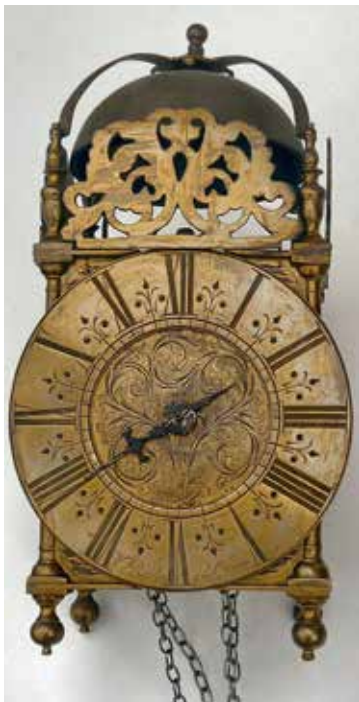
Figure 5. Lantern clock of the 1690s by William Barlow of King's Lynn made originally with a verge pendulum swinging between the trains but converted later to anchor escapement. The original broken hand has been repaired wrongly.
