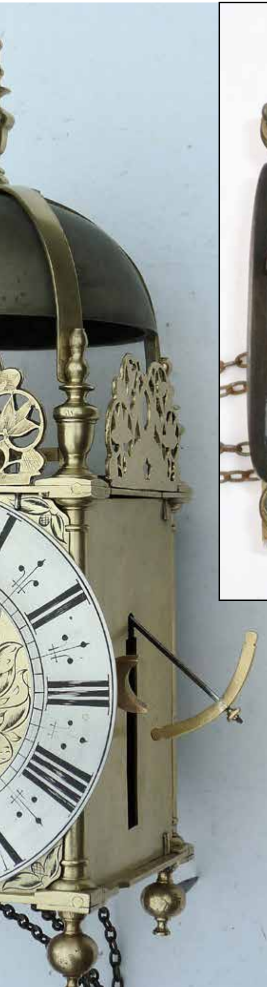
Figure 3 (left). This angled view from the right with the door closed shows how the anchor-shaped pendulum fluke swings through the slot. The angle of swing is exaggerated in the photograph. This type of centre pendulum lantern clock sometimes had 'wings', but not all, as evidenced by this one.
