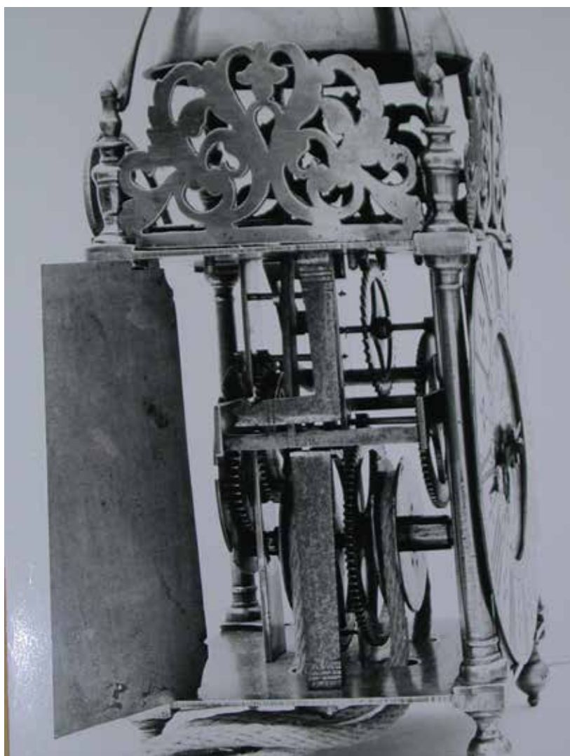
Figure 7. Movement of the lantern clock by John Risbridger. By now the movements were plainer with less decorative filework.
