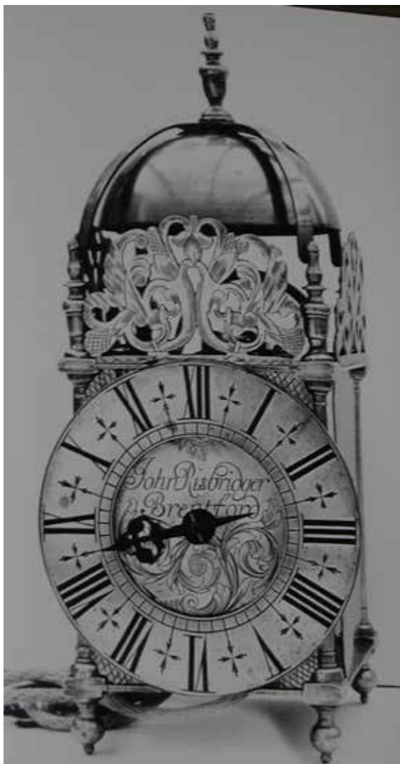
Figure 6. Lantern clock of about 1710-1720 by John Risbridger of Brentford, with original anchor escapement.
