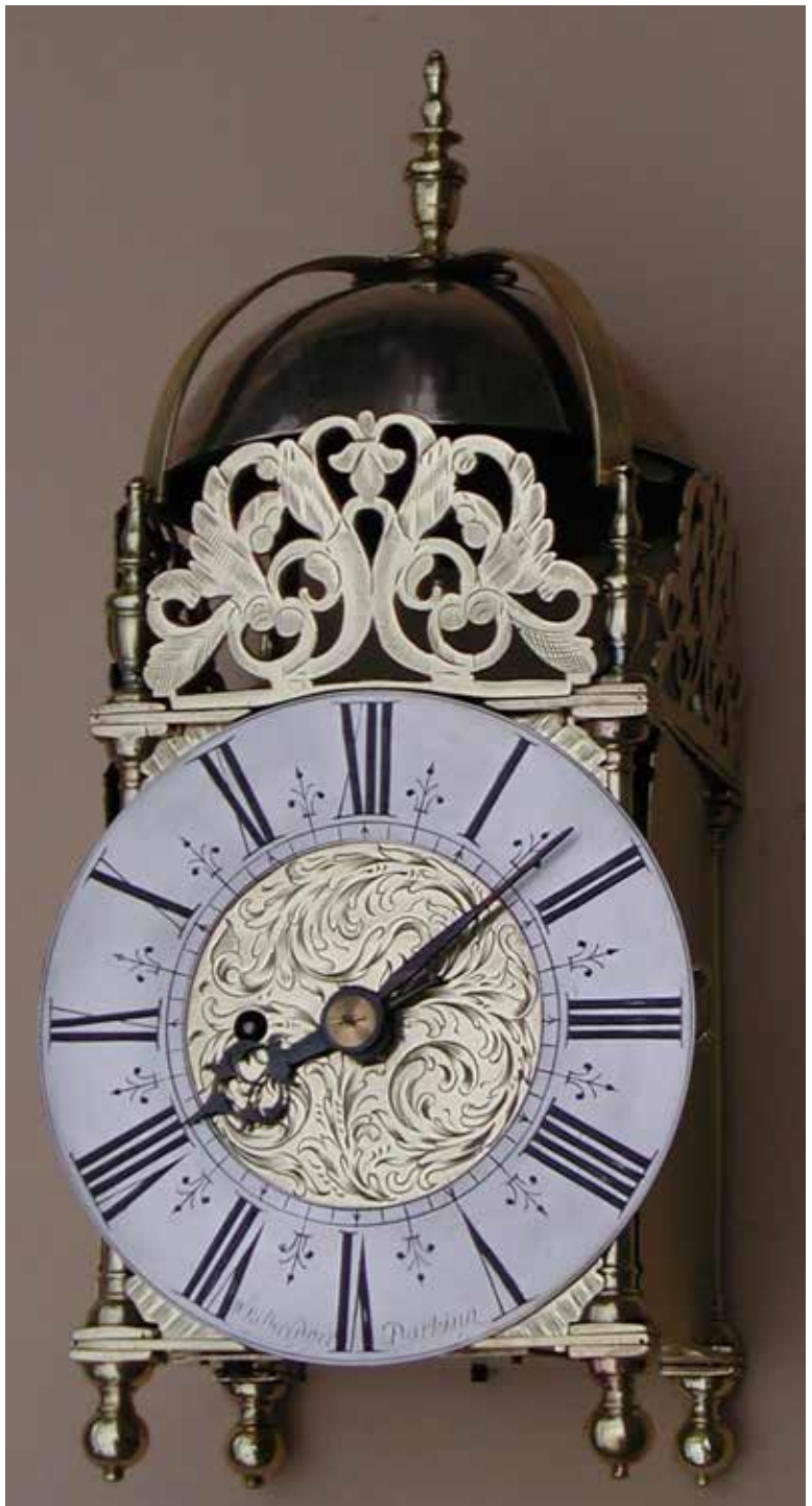
Figure 5. Lantern clock by William Risbridger (I) of Dorking dating from 1690-1700. This example was converted later to two hands and was fitted with a later spring-drive movement.
