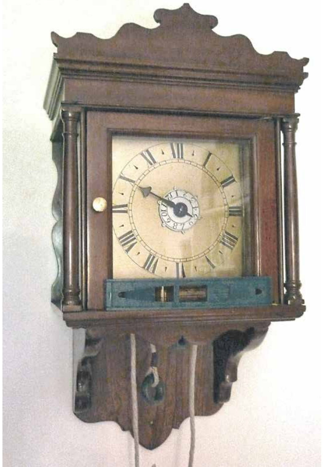
Figure 4 (right). The best place to position a spirit level is in front of the glass hood door. This example is a hooded clock. It is even more important to set a wall clock level than a longcase as any lean from vertical will be more apparent.
