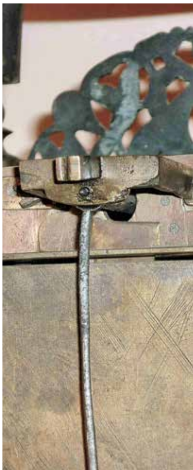
Figure 14. Back view of the clock showing the experimental back cock and crutch fitting.
