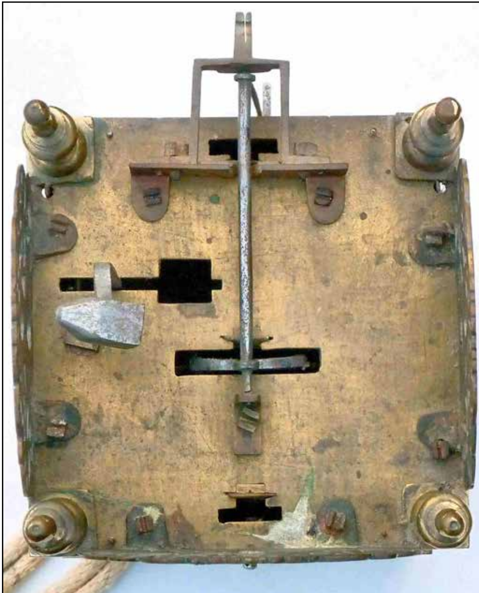
Figure 13. The top view shows the extraordinary use of a longcase pendulum back cock adapted to make it fit on to the top plate. Evidence of experimentation?
