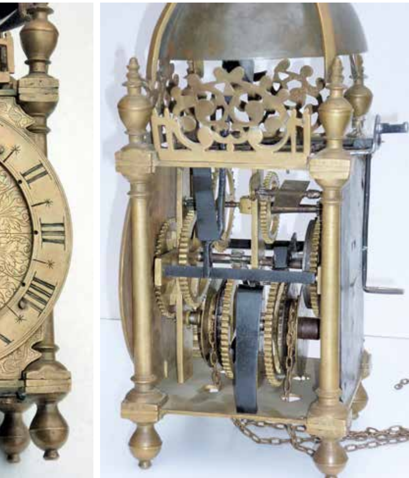
Figure 5. The movement seen from the right shows the conversion to anchor escapement. The straight hammer counter is a very early feature.
