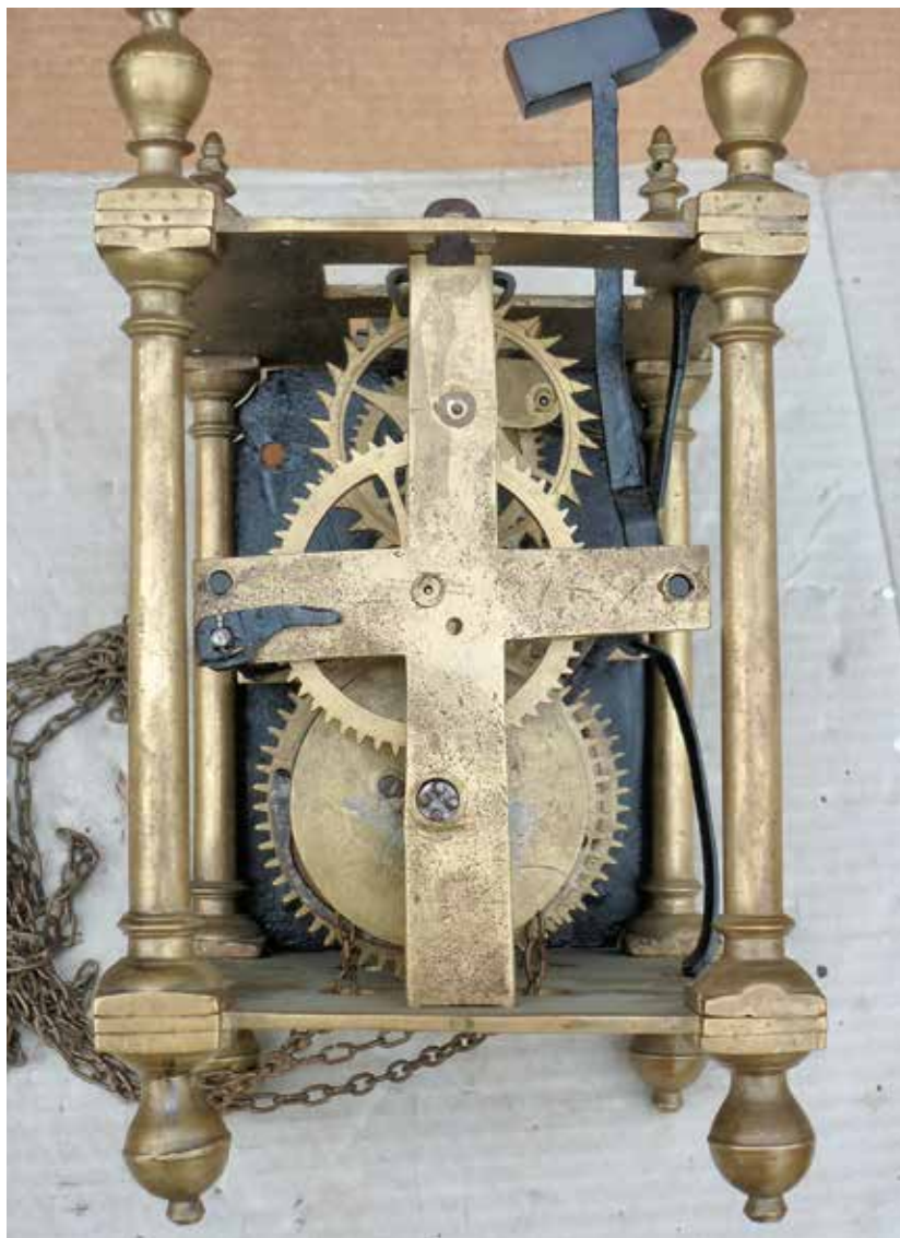
Figure 12. The dial removed to show the movement. The crossbar, which carries the two strike detent arbors (on the left in this view), does not need filing back at the front, as it does at the back (seen in figure 6).
