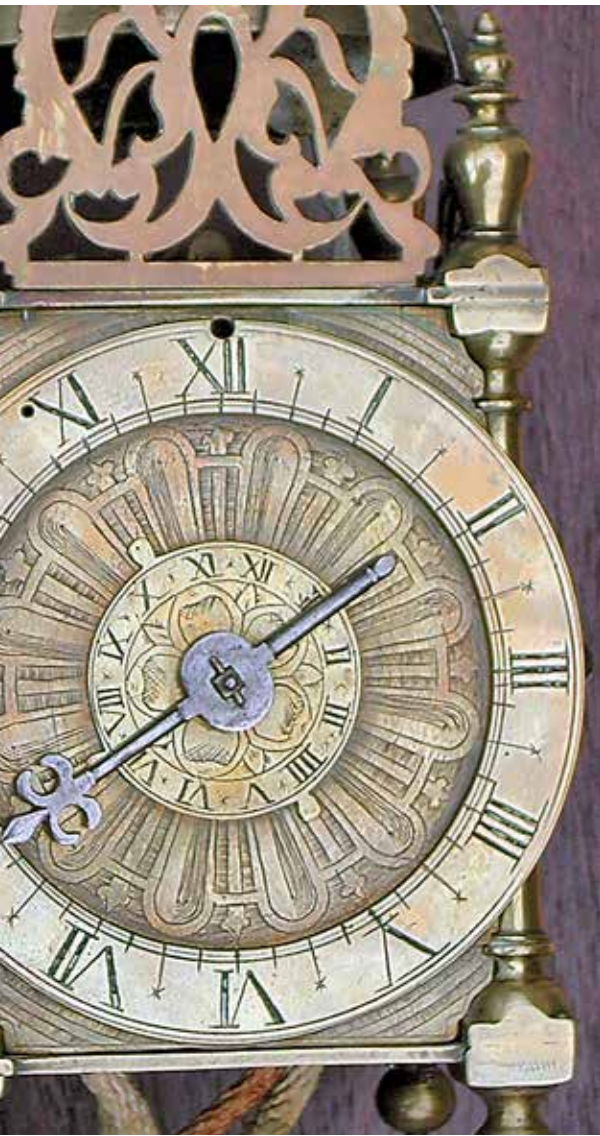
Figure 13. This early unsigned gadrooned clock from the Harvey workshop has the dial attached by a screw above 'XII', a characteristic feature used later only by Henry Stevens on his signed clocks. Front fret replaced later.
