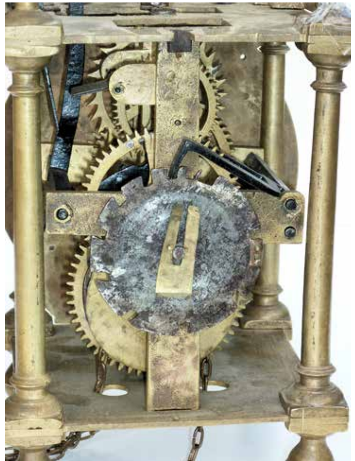
Figure 6. The rear view shows the iron countwheel and the distinctive filed cutback in the crossbar arm to allow the strike levers to return. The strike fly, originally positioned in the main crossbar, has been re-positioned to one side to avoid it catching the anchor arbor after conversion to pendulum.
