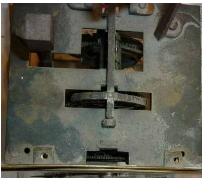
Figure 6. The maker had to re-position his dial attachment lugs, otherwise as first planned their riveted ends would have shown in the dial centre instead of being hidden behind the chapter ring, as now, evidence that the maker was inexperienced at this time.
