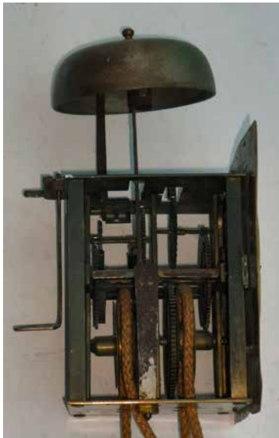
Figure 4. Left view of the posted movement. The ironwork is painted black, or 'japanned' to prevent rust. This was often done by restorers after servicing, but it is not known whether this was also sometimes done at the time of making.
