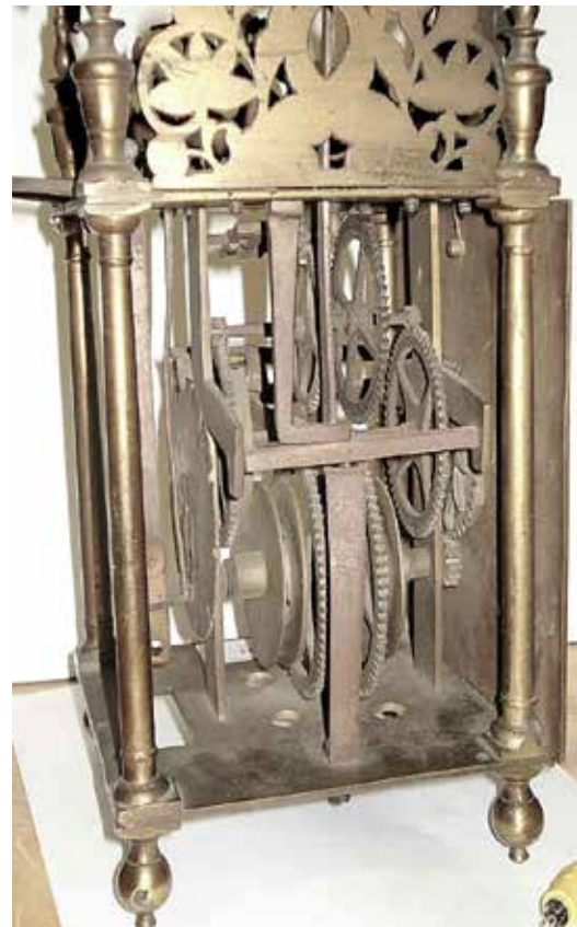
Figure 3. The movement is pictured here before cleaning. It was made with a verge pendulum and was converted to long pendulum at a later date.
