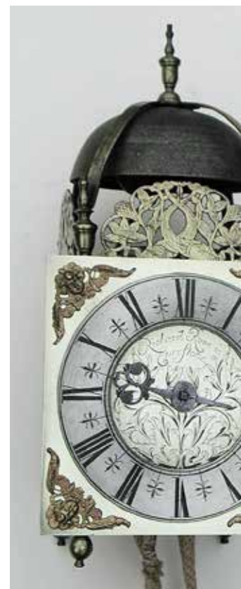
Figure 9. Quaker clockmaker Richard Roe of Epperstone in Nottinghamshire made this 7in (18cm) dial verge-pendulum lantern clock about 1690. His dial engraving is based on earlier London styling but develops into his own design.
