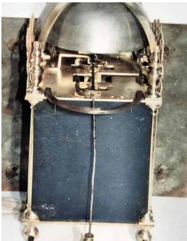
Figure 7. The rear view of this clock shows its verge pendulum. It has full lantern clock features such as hoop, spurs, doors and frets
