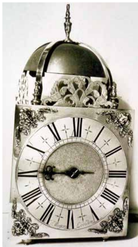
Figure 8. This verge-pendulum lantern clock by John Mason of London has an 8in (20cm) dial and dates from about 1690-1700.
